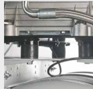
Engine/unit base installed on 4 anti-vibration rubber dampers for less vibrations, reduced noise and longer service life (only on Diesel models)
